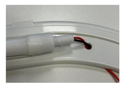
7. Refit rubber LED strip to clear plastic lens
