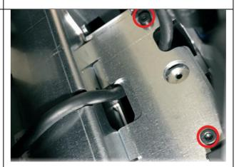
Finally, locate and place the cable cover, and the last hex head retaining bolt.
