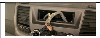
2 Using trim removal tools, carefully release the dashboard fascia panel.
