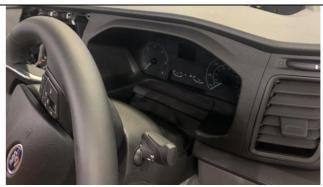
With the surround removed, remove the 4 x screws securing the cluster in place. Once the cluster is free, pull forward from its location, disconnect the plug from the rear and store safely.
