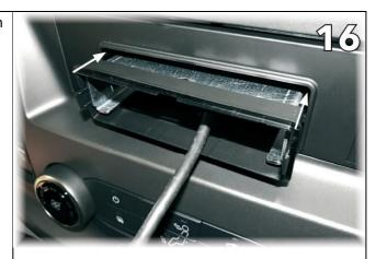
Locate the display assembly. Connect the display cable. Slide the brackets from the display assembly into the main unit and secure with the provided hex head bolts.
