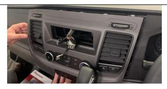
3 Using trim removal tools, carefully unclip and release the instrument cluster surround. Once the surround has been release, carefully maneuver it free from its position
