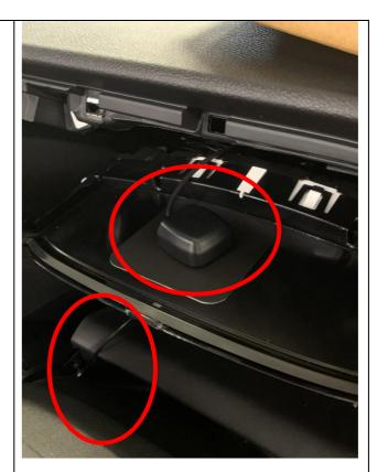
Begin to locate the cluster surround into position. Ensure that the microphone exits between the rear of the surround and the face of the cluster as shown.
