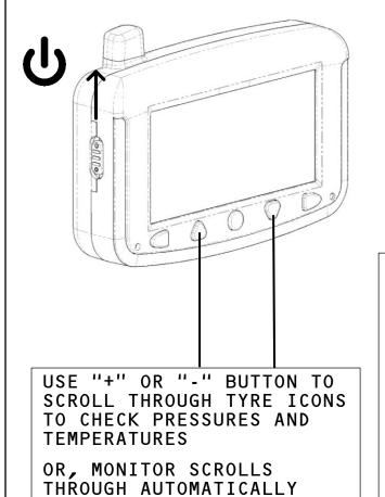
THE MONITOR DOES NOT NEED A PERMANENT POWER SUPPLY FROM THE VEHICLE TO FUNCTION. THE INTERNAL BATTERY PROVIDES APPROX. 60 HOURS OF CHARGE.
