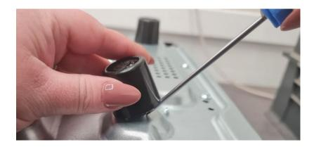
2. Remove the rivet pin from the foot:
