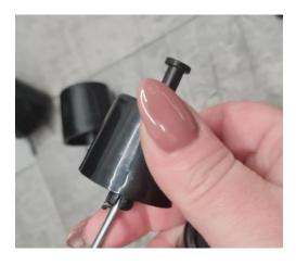
3. Carefully cut the barbs off flush with the top of each foot.
