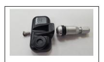
Unscrew the old valve from the sensor.
