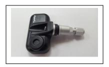
Screw the valve onto the exposed thread and hand tighten as much as possible.
